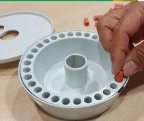
The Adama InJecta magazine is designed to hold 30 Di-bak capsules and sealing plugs. These are loaded in tandem into each of the 30 chambers. Note that the magazine has 31 chambers as one (in central position) must remain empty to allow for the initial drilling action. The inner section rotates in a clockwise direction.
